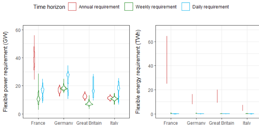
Figure 3: Flexibility requirements for different timescales and different countries. Electric heating and cooling levels are at 2017 levels, VRES generation has not been deduced from the load, interconnection has not been taken into account.
