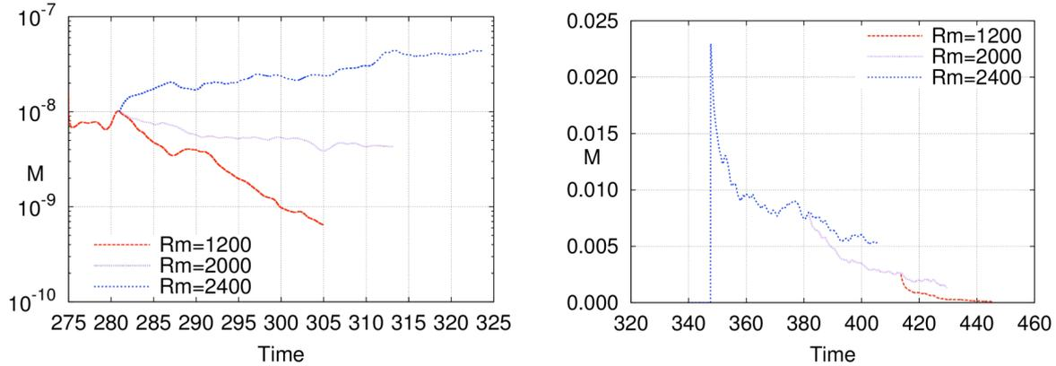
Figure 4: Time evolution of the magnetic energy  $M$  in the conducting fluid (left) in the linear regime from  $t=275$  at  $Re=1200$  and various  $Rm$  as indicated (in lin-log scale) and (right) in the nonlinear regime for  $Re=1200$  and various  $Rm$  as indicated. *Equatorial spin* case.
