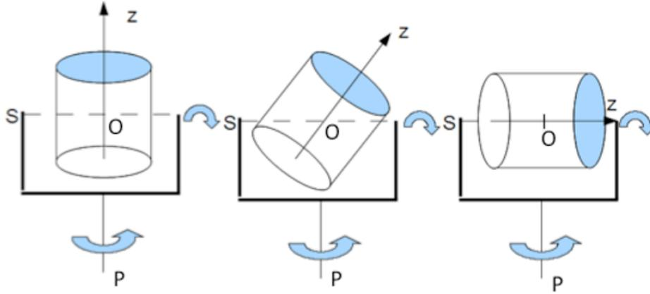
Figure 1: Different ways of spinning for precession driving: (left) equatorial spin (the spin angle is  $\pi/2$ ); (middle) oblique spin; (right) axial spin (the spin angle is 0). OS is the spin axis, OP the precession axis and Oz the symmetry axis.
