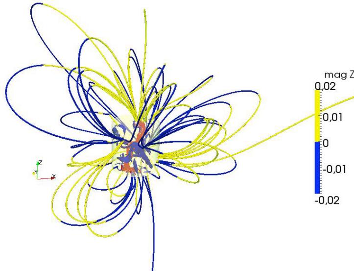
Figure 5: Snapshot at  $Re=1200$  and  $Rm=2400$  of the vorticity field lines (grey/red) and the magnetic field lines colored by the axial component (light grey/yellow for positive vertical magnetic field component and black/blue for negative vertical magnetic field component). The view is seen from the side ( $Ox$  is the spin axis,  $Oz$  the precession axis). *Equatorial spin* case.
