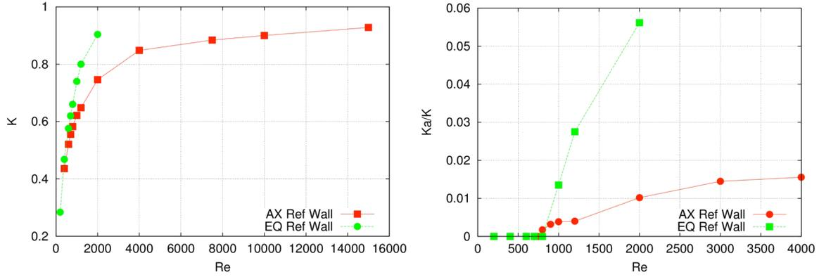
Figure 2: Comparisons between the axial and equatorial spin cases in the reference frame of the wall (also called the *mantle frame*) for a fixed precession rate 0.15: (left) total kinetic energy as a function of  $Re$ ; (right) asymmetry ratio  $Ka(t)/K(t)$  as a function of  $Re$ .
