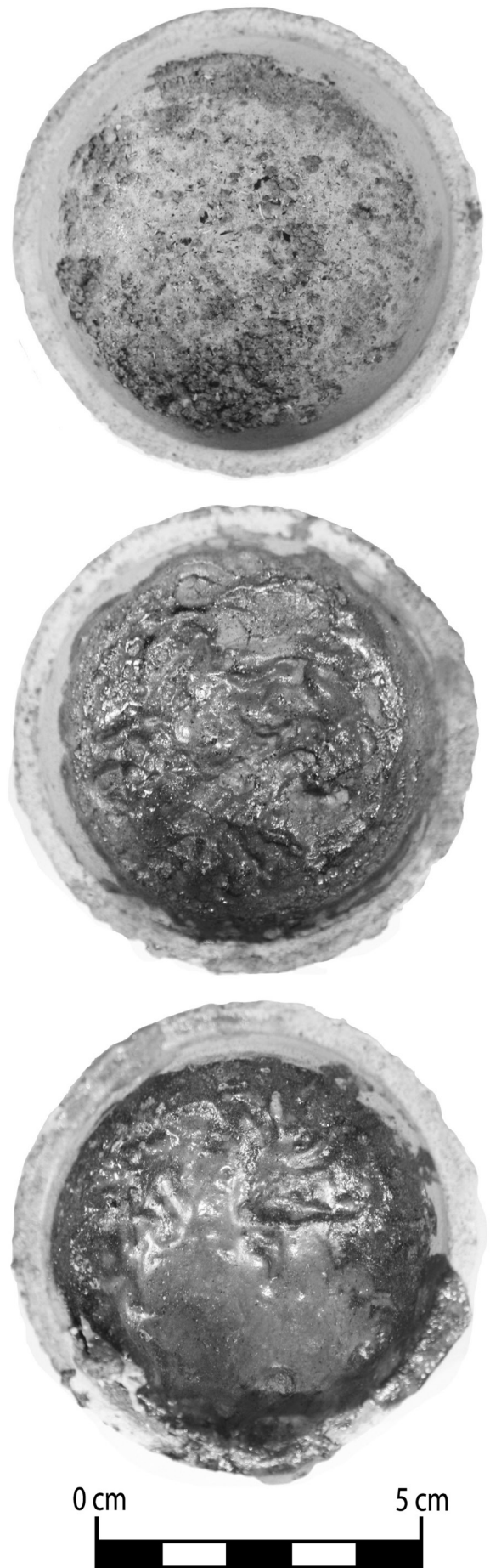
Figure 7: Scorifiers after three assays of one Italian sample: the first without additional lead, the second with two parts of lead, the third with four parts of lead.
