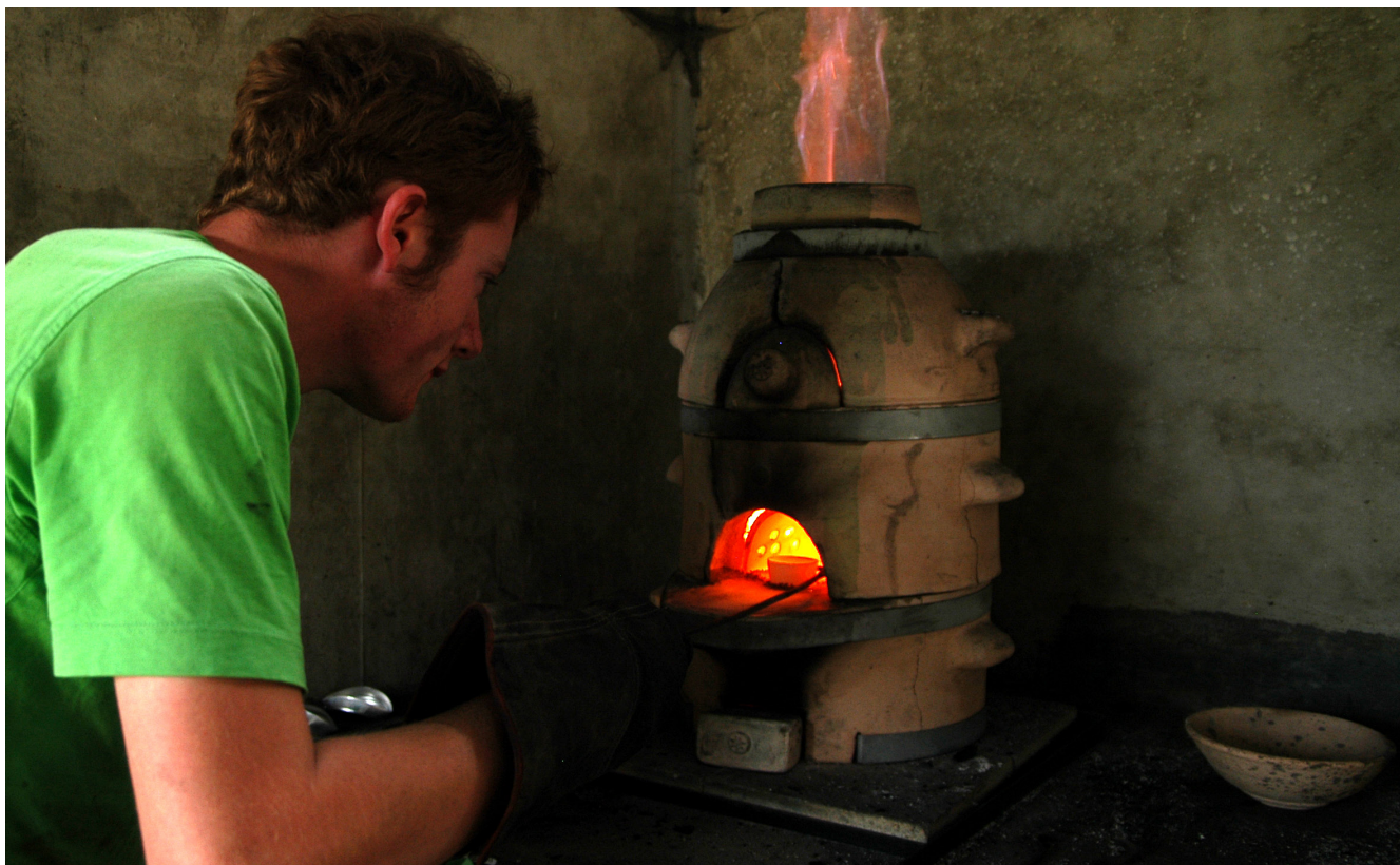
Figure 1: The muffle furnace used for the experiments.
