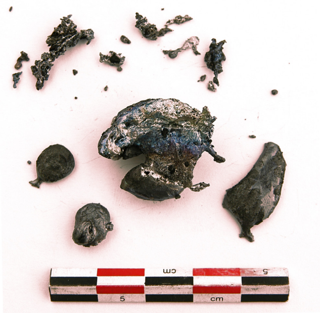
Figure 6: Result of an assay with charcoal slack addition: the regulus is fragmented.
