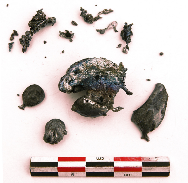
Figure 6: Result of an assay with charcoal slack addition: the regulus is fragmented.
