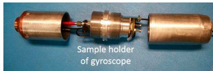
Figure 19. Test vehicle accelerated by electromagnetic force to generate high shocks.
