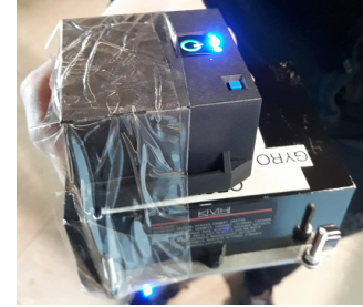
FIG. 5 –. The additional mass taped to ULISS device.
