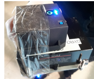
FIG. 5 –. The additional mass taped to ULISS device.
