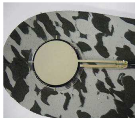
Figure 3. A401 sensor and its electronic conditioning
