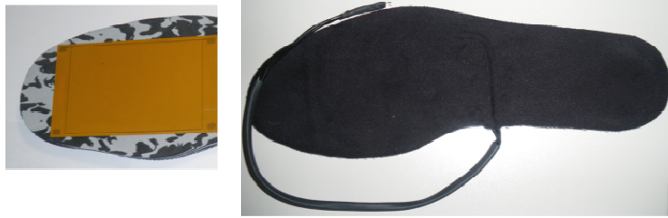
Figure 17. Integration of the MFC-M8557P2 generator
