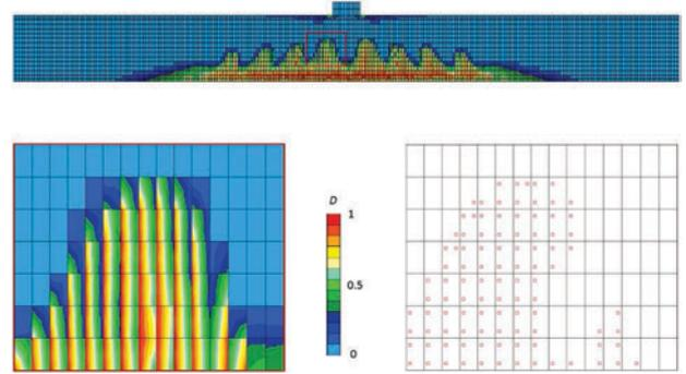
**Figure 3.** Damage distribution in a three points beam test (top figure). Zoom on damage oscillation problems (left figure) and loading integration points (red rectangles correspond to integration points with an increasing damage variable, right figure)
