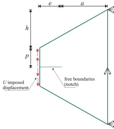
**Figure 11.** Notched trapezoidal beam: mode I crack propagation test<sup>46</sup>
