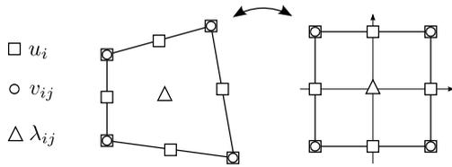
Figure 1. The 2D second gradient finite element<sup>36</sup>
