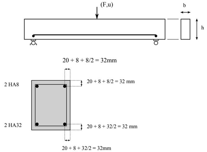
**Figure 2.** Three points bending test: beam dimensions and steel reinforcement<sup>43, 44</sup>
