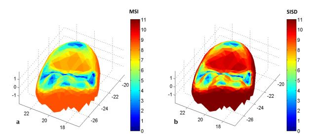
**Figure 3**: Case study 1. Predicted SI performance indicators maps with VITA Enamic biomaterial and lyra bur at a milling feed rate of F2000 mm/min. (a) MSI predicted SI performance indicator map. (b) SISD predicted SI performance indicator map.
