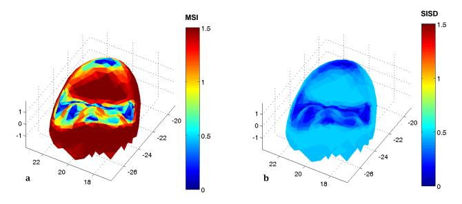
**Figure 4**: Case study 2. Predicted SI performance indicators maps with VITA Enamic biomaterial and lyra bur at a milling feed rate of F2000 mm/min. (a) MSI predicted SI performance indicator map. (b) SISD predicted SI performance indicator map.
