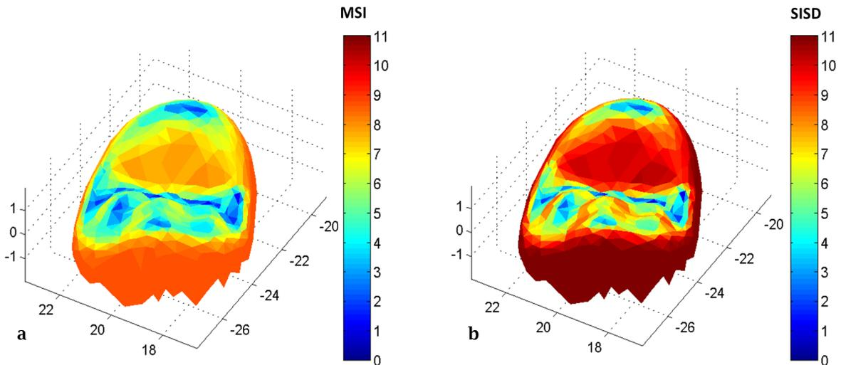
**Figure 3:** Case study 1. Predicted SI performance indicators maps with VITA Enamic biomaterial and lyra bur at a milling feed rate of F2000 mm/min. (a) MSI predicted SI performance indicator map. (b) SISD predicted SI performance indicator map.
