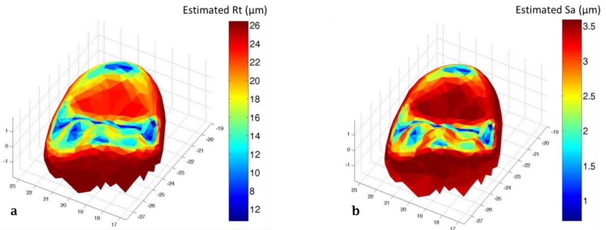
**Figure 2:** Predicted roughness maps with VITA Enamic biomaterial and lyra bur at a milling feed rate of F2000 mm/min. (a) Rt 2D roughness predicted map. (b) Sa 3D roughness predicted map.
