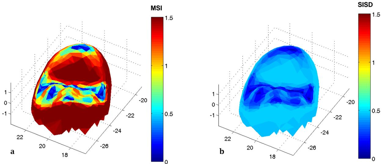
**Figure 4:** Case study 2. Predicted SI performance indicators maps with VITA Enamic biomaterial and lyra bur at a milling feed rate of F2000 mm/min. (a) MSI predicted SI performance indicator map. (b) SISD predicted SI performance indicator map.
