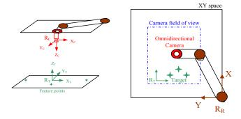
Fig. 5. 3-dof planar manipulator
