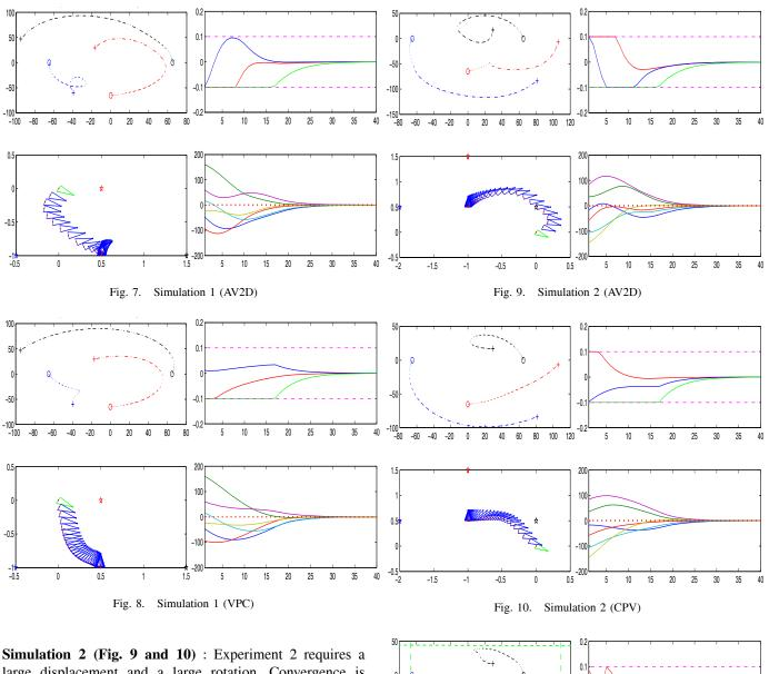
**Simulation 2 (Fig. 9 and 10)**: Experiment 2 requires a large displacement and a large rotation. Convergence is obtained for both controllers. The VPC results (Fig. 10) are clearly better. The camera trajectory in the XY space and the feature trajectories in the image plane are optimal.
