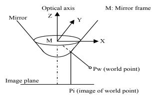
Fig. 6. Point projection: parabolic mirror and orthographic camera
