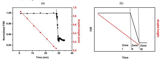
Fig. 1 (a) Experimental plot of the free spectral range and the height of the droplet against time during the drying of a 10  $\mu$ L sessile droplet at T = 24 °C. (b) Generic shape of the FSR and droplet height dynamics during a drying process.
