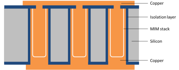
Fig. 17. Schematic representation of fully through going TSCs component in silicon interposer.
