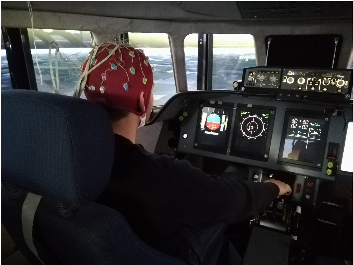
Figure 3. ISAE-SUPAERO three axis motion flight simulator. The participants were left seated and equipped with a Biosemi 32-electrode EEG system.
