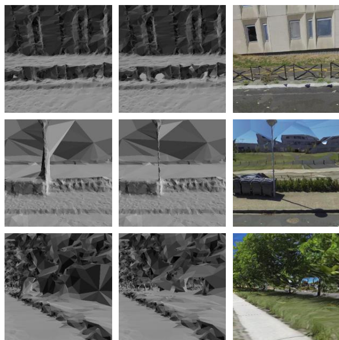
Figure 21: Varying \alpha for the method M3: \alpha = 0.3 on the left and \alpha = 0.1 on the middle and right. There are views of a fence in front of a building, a light post between two streets, and tall grass under trees.
