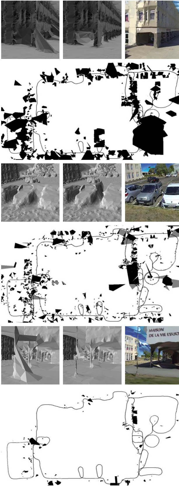
Figure 18: Improvements done by C.E.R (top), S.G. (middle) and C.H.R. (bottom) involved in method M2. In each case, there is a top view of tetrahedra switched from F \setminus O to O (in black) or from O to F \setminus O (in grey, S.G. only), superimposed by the camera trajectory. There are also local views of the surface obtained without and with the operation.
