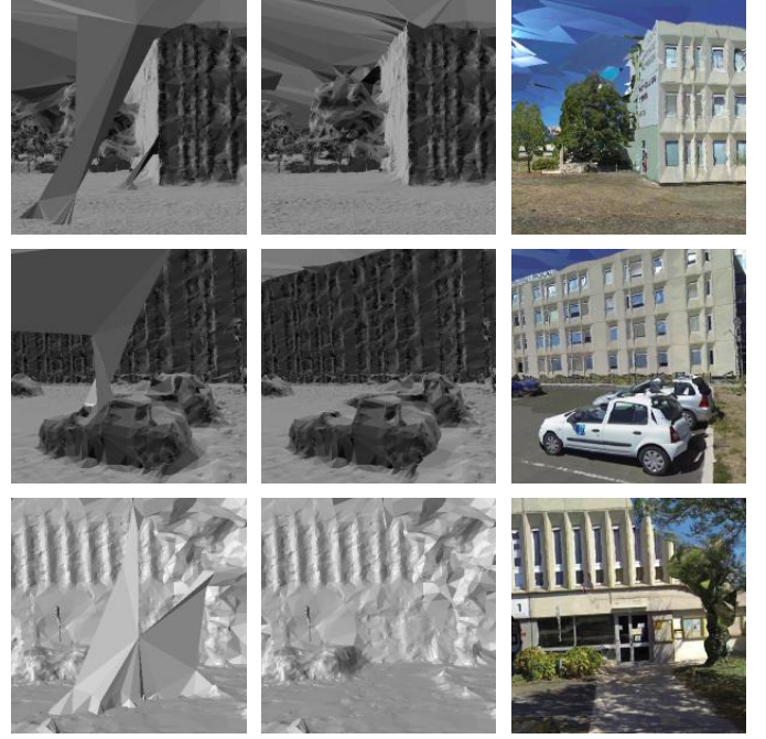
Figure 15: Examples of removals of spurious handles by [22] without (left) and with (middle and right) C.H.R. involving Repair2.
