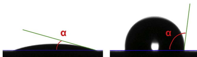
Fig. 4. Example of pictures used for contact angle measurement. Left: reference sample, \alpha = 19.6^\circ ; right: sample with initial concentration of Bio-Terge of 25 g/L, \alpha = 103^\circ .
