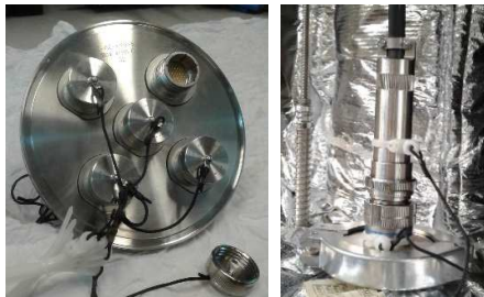
Fig. 3: 300K feedthroughs from the production (left) and 80K feedthrough prototype with its connectors (right)
