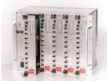
Fig. 1: ITER's 19" crate with five CABTR boards (40 channels)
