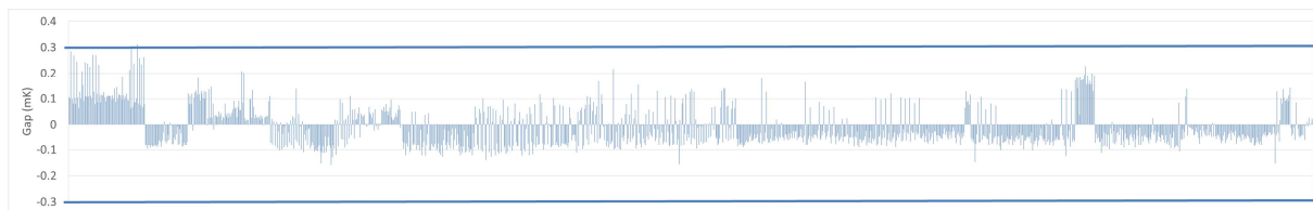
Fig. 9: Results @77K for produced thermo-blocks after five LN 2 cycles on CYTROGEN test bench - IO’s criteria: \pm 300\text{mK}
