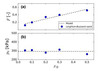
**Fig. 6** a The evolution of F, the maximum deformed fraction of rubber, is affine with  $x_R$  in the studied range of  $x_R$  ( $F = 0.1 + 0.95 x_R$ ). **b** In contrast, the pressure  $p_0$  characterizing the exponential decay of the void ratio versus the applied pressure is almost constant with the volume ratio of rubber ( $p_0 \approx 296.6 \text{ kPa}$ )
