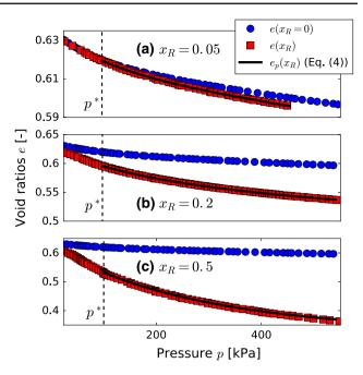
**Fig. 5** Comparison between experimental void ratios and those obtained by our model for several volume ratios of rubber and the Leighton Buzzard sand for  $\mathbf{a}$   $x_R = 0.05$ ,  $\mathbf{b}$   $x_R = 0.2$  and  $\mathbf{c}$   $x_R = 0.5$ . Squares (resp. circles) correspond to the sample with rubber  $(e(x_R, p))$  (resp. without rubber  $e(x_R = 0, p)$ ) and the solid line to the prediction of our model  $e_p(x_R, p)$ . As in Fig. 4, the vertical dashed line corresponds to  $p = p^*$
