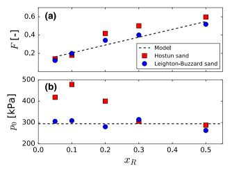
**Fig. 9** a The maximum deformed fraction of rubber, F, depends weakly on the type of sand (Leighton Buzzard or Hostun RF) and  $F_{model}$  captures correctly the experimental values obtained with Hostun RF sand. b The characteristic pressure depends on the type of grains for  $x_R < 0.3$ . Above this value, the behaviour of the mixture is rubber-like, and  $p_0$  becomes independent of the rubber volume fraction
