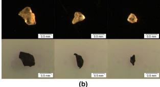
Fig. 3 Individual particles of sand (top) and equivalent rubber chip particles (bottom) for  ${\bf a}$  the Leighton Buzzard sand and  ${\bf b}$  the Hostun RF sand
