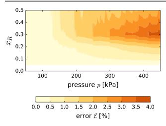
**Fig. 8** The error between the prediction of our model and the experimental results for Hostun RF sand–rubber is maximum for a rubber ratio approximatively equal to 0.3 and important pressures ( $p \approx 450 \text{ kPa}$ )
