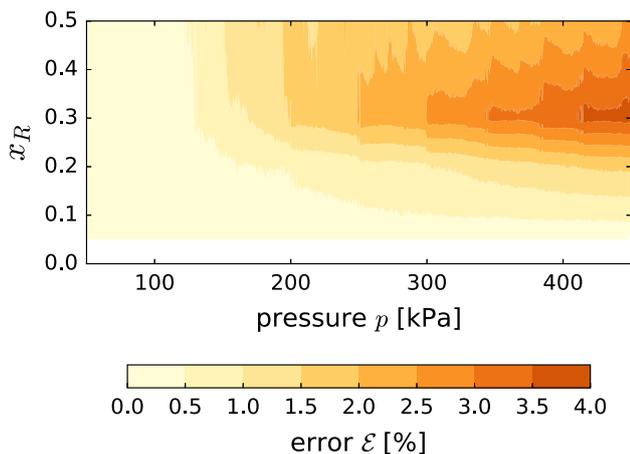
**Fig. 8** The error between the prediction of our model and the experimental results for Hostun RF sand–rubber is maximum for a rubber ratio approximately equal to 0.3 and important pressures ( $p \approx 450$  kPa)
