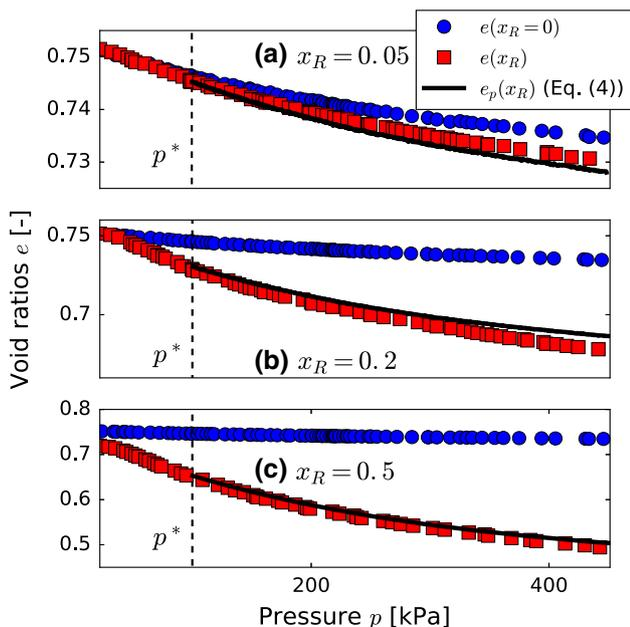
**Fig. 7** Comparison between experimental void ratios and those obtained by our model for several volume ratios of rubber and the Hostun RF sand for **a**  $x_R = 0.05$ , **b**  $x_R = 0.2$  and **c**  $x_R = 0.5$ . Squares (resp. circles) correspond to the sample with rubber ( $e(x_R, p)$ ) (resp. without rubber  $e(x_R = 0, p)$ ) and the solid line to the prediction of our model  $e_p(x_R, p)$ . As in Fig. 5, the vertical dashed line corresponds to  $p = p^*$
