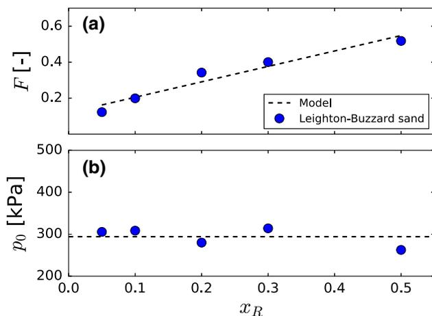
**Fig. 6** **a** The evolution of  $F$ , the maximum deformed fraction of rubber, is affine with  $x_R$  in the studied range of  $x_R$  ( $F = 0.1 + 0.95 x_R$ ). **b** In contrast, the pressure  $p_0$  characterizing the exponential decay of the void ratio versus the applied pressure is almost constant with the volume ratio of rubber ( $p_0 \approx 296.6$  kPa)
