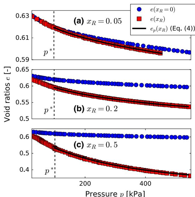
**Fig. 5** Comparison between experimental void ratios and those obtained by our model for several volume ratios of rubber and the Leighton Buzzard sand for **a**  $x_R = 0.05$ , **b**  $x_R = 0.2$  and **c**  $x_R = 0.5$ . Squares (resp. circles) correspond to the sample with rubber ( $e(x_R, p)$ ) (resp. without rubber  $e(x_R = 0, p)$ ) and the solid line to the prediction of our model  $e_p(x_R, p)$ . As in Fig. 4, the vertical dashed line corresponds to  $p = p^*$
