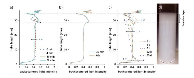
**Figure S6.** a) to c) Evolution with time of the curves of the backscattered intensity versus tube height for an emulsion of PLGA-PVA NP suspension at 25 mg/mL and Miglyol (ratio 90-10). Example of a) a creaming stage b) a stability stage c) a coalescence-flocculation stage. d) Image at D7 of an emulsion containing 10% (w/w) of Miglyol and 90% (w/w) of lyophilized PLGA-PVA NP suspension at 25 mg/mL in water.
