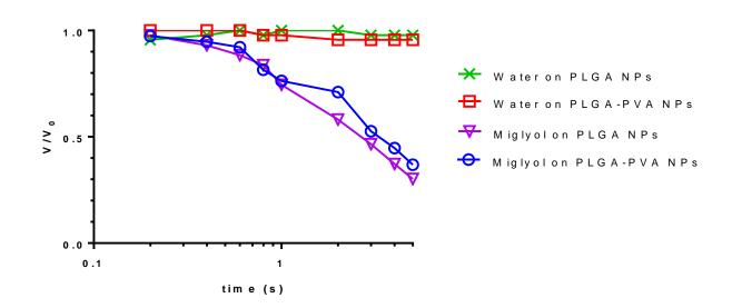
**Figure S5.** Evolution with time of the droplet volume ratio  $V/V_0$  deposited on a dense PLGA NP or PLGA-PVA NP layer. V is the droplet volume and  $V_0$  is the droplet volume at t = 0.
