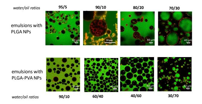
**Figure S8.** Confocal microscopy images of emulsions (green channel: aqueous phase; red channel: NPs) for different water/oil ratios. Oil phase (Miglyol) was not colored and appeared in black.
