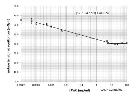
**Figure S11.** Plot of the surface tension at equilibrium versus PVA concentration in order to determine the CAC of PVA.
