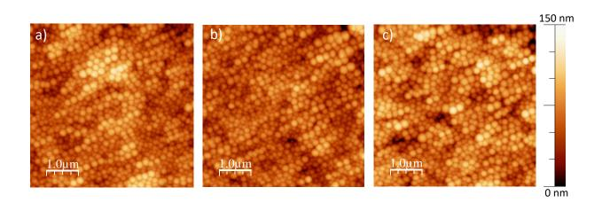
**Figure S4.** Topographic AFM Images (5.0 μm x 5.0 μm) of dried NPs layer of a) PLGA-PVA NPs b) lyophilized PLGA-PVA NPs and c) PLGA NPs.
