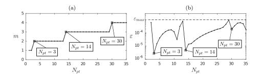
Figure 3: Beam with cubic spring – (a) Number of PGD modes m and (b) error measure  $\varepsilon$  against point index  $N_{\rm pt}$ .
