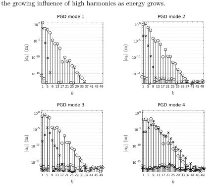
Figure 5: Beam with cubic spring – Amplitudes of (cosine) Fourier coefficients of PGD modes. Crosses: coefficients when the mode is first introduced; Circles: coefficients at the end of the branch ( $N_{\rm pt} = 35$ ).
