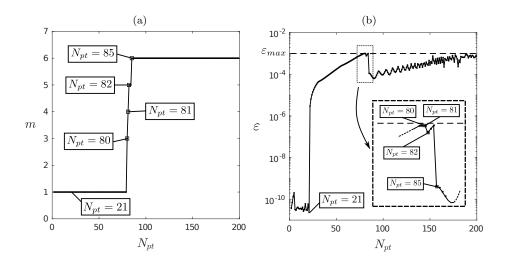
Figure 7: Beam with unilateral contact – (a) m and (b) residue  $\varepsilon$  against  $N_{\rm pt}$ . Dotted line: convergence threshold.
