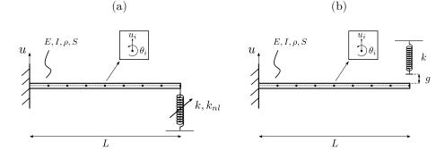
Figure 1: Euler-Bernouilli cantilever beam (a) with a transverse cubic spring at dof 1 (b) with a transverse gap between dof 1 and the linear spring.
