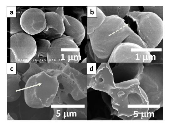
**Figure 10.** SEM micrographs of the PSt beads (a, b) and cryo-fractured PBuA beads (c, d) obtained after PEII-AGET-ATRP polymerization of the emulsions, performed without sacrificial initiator. The dashed arrow points at an empty CNC-g-PSt capsule; the plain arrow points at a plain CNC-g-PBuA bead (cut in half by cryo-fracture).
