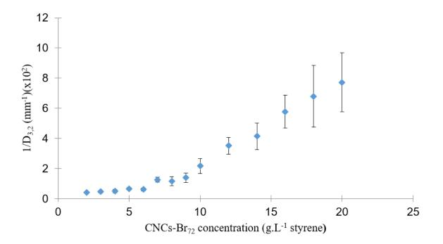
Figure 4. Evolution of the reciprocal Sauter's diameter of the W/O emulsion droplets as a function of CNC-Br<sub>72</sub> concentration (W/O ratio = 57/43 v/v).
