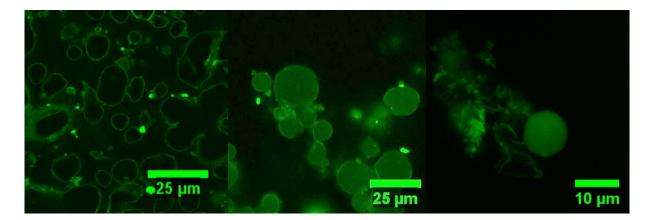
**Figure 11.** Laser confocal fluorescence microscopy of the O/W *n*-BuA emulsion stabilized by the FC-CNC-Br<sub>4</sub> particles, before (left), during (center) and after (right) polymerization (O/W ratio: 1/9 v/v; 5g/L FC-CNC-Br<sub>4</sub>, 5g/L CNCAs<sub>9</sub>).
