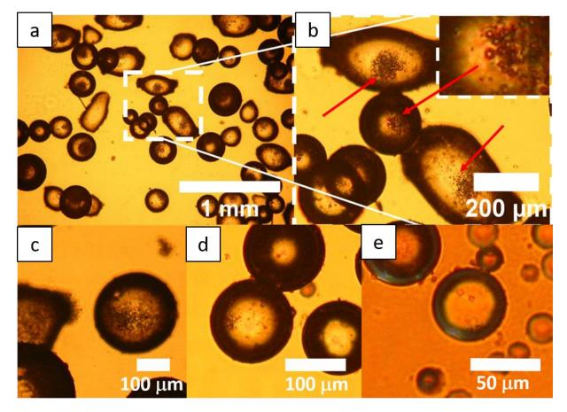
**Figure 5.** Optical micrographs of the invert W/O stabilized by (a, b, c)  $2 \text{ g.L}^{-1}$  (d)  $5 \text{ g.L}^{-1}$  and (e)  $12 \text{ g.L}^{-1}$  of CNC-Br<sub>72</sub>.
