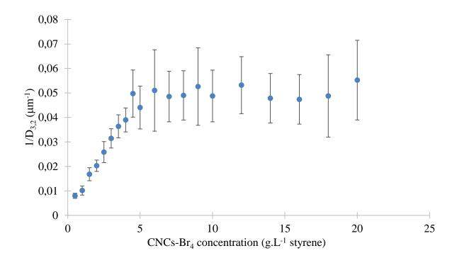
**Figure 3.** Evolution of the reciprocal Sauter's diameter of the O/W St emulsion droplets as a function of CNC-Br<sub>4</sub> concentration (O/W ratio =10/90 v/v). The error bars represent the emulsion polydispersity.
