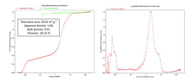
**Figure 13.** Cumulative intrusion (expressed as cumulative intrusion vs applied pressure) (left) and pore size distribution (expressed as Log differential Intrusion vs pore size) (right) in the polymerized inverted W/O St emulsion measured by mercury porosimetry.
