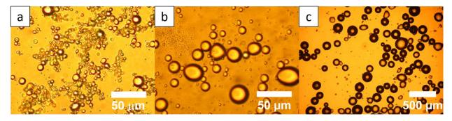
**Figure 2.** Optical micrographs of the direct O/W (a, b) or inverted W/O (c) St emulsions stabilized with a) CNC-Br<sub>1</sub>, b) CNC-Br<sub>4</sub> and c) CNC-Br<sub>72</sub> (O/W ratio =10/90 v/v; 5g CNC-Br /L of St).
