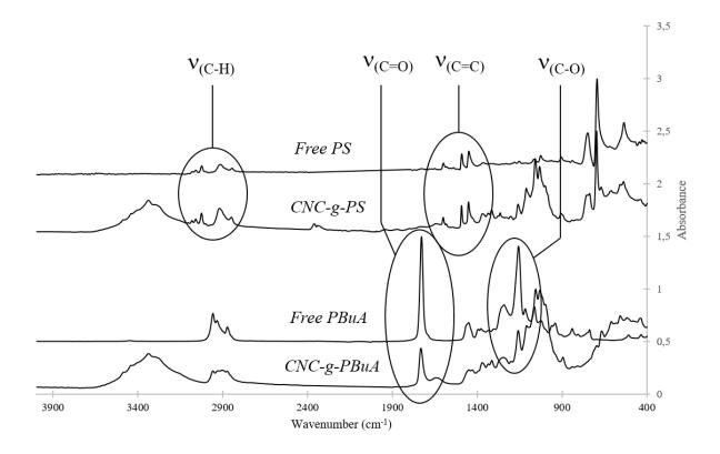
**Figure 9.** FT-IR spectra of the solid material remaining after the THF extraction (CNC-g-PSt and CNC-g-PBuA), and free polymers recovered (PSt and PBuA) after elimination of the solvent.
