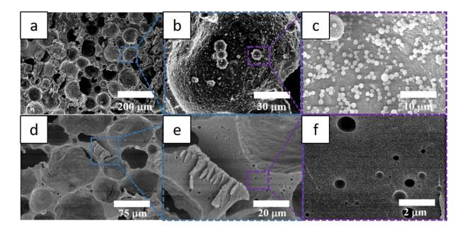
**Figure 12.** SEM micrographs of the PSt material obtained after PEII-AGET-ATRP polymerization of the inverted W/O St emulsion stabilized by the CNC-Br<sub>72</sub> particles. The macroporosity M<sub>1</sub> (a
