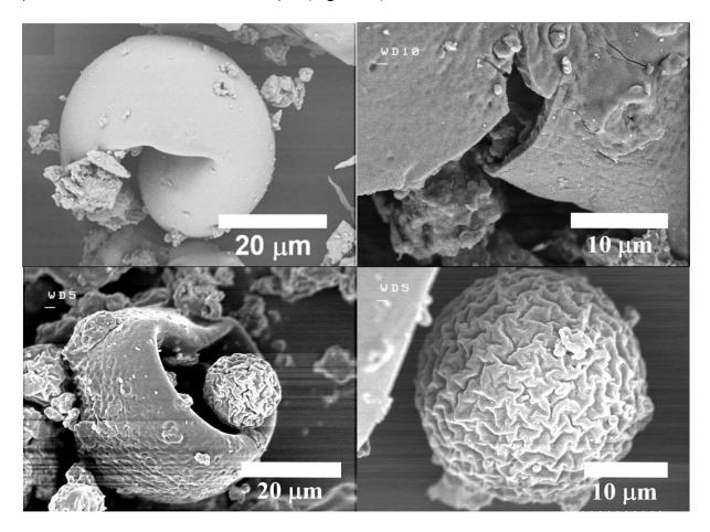
**Figure 14.** SEM micrographs of the PSt material obtained after PEII-AGET-ATRP polymerization of the multiple W/O/W St emulsion stabilized by CNC-Br<sub>72</sub>, CNCAs<sub>9</sub> and CNC-Br<sub>4</sub> particles. Capsules and inner polymerized beads with PSt coagula can be seen.
