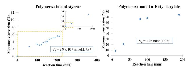
**Figure 8.** Kinetics of the PEII-AGET-ATRP polymerization of styrene (left) and *n*-butyl acrylate (right), followed by <sup>1</sup>H NMR.
