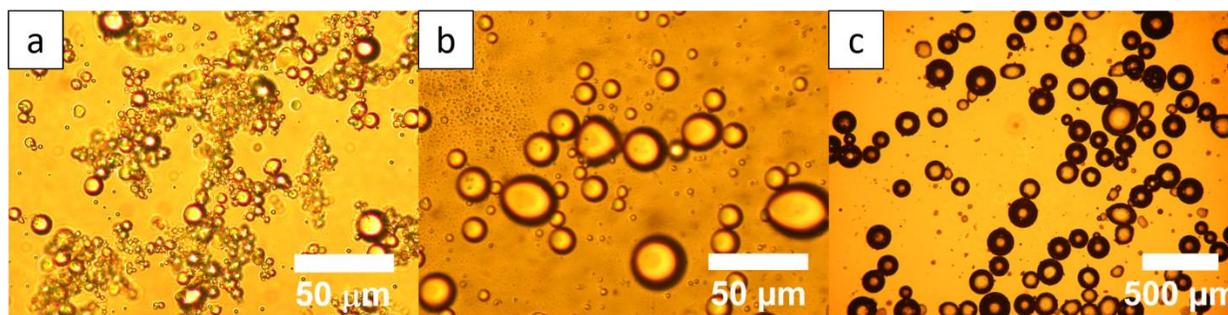
**Figure 2.** Optical micrographs of the direct O/W (a, b) or inverted W/O (c) St emulsions stabilized with a) CNC-Br<sub>1</sub>, b) CNC-Br<sub>4</sub> and c) CNC-Br<sub>72</sub> (O/W ratio =10/90 v/v; 5g CNC-Br /L of St).
