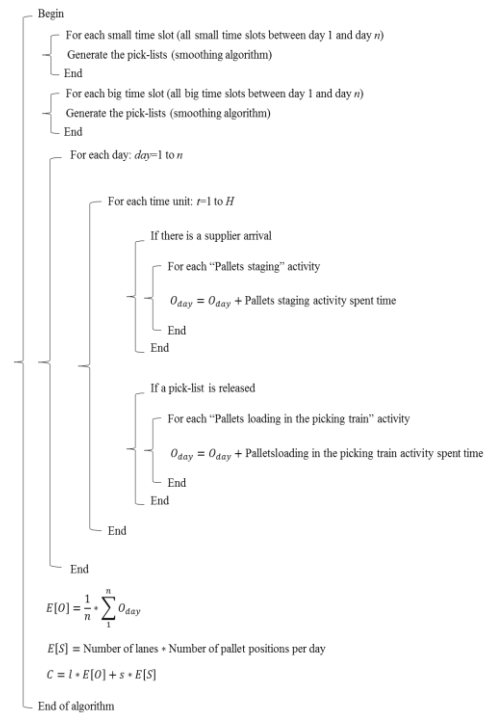
Algorithm 1. Algorithm of calculation of cross-docking cost
