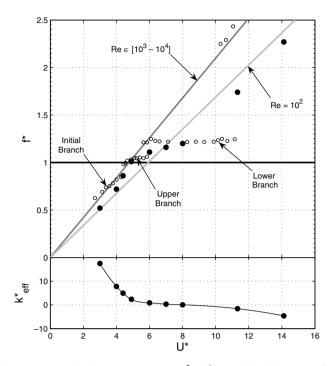
Fig. 19. Reduced frequency response  $f^* = f/f_H$  and lock-in zone. (•) Present simulation, ( $\bigcirc$ ) [22]. The black line indicates the oscillation at  $f_H$  whereas the gray lines correspond to oscillations at the Strouhal frequency for the range of Reynolds number considered. The subplot give the correspondence between the parameters  $k_{eff}^*$  and  $U^*$  used respectively by Shiels et al. [40] and Khalak and Williamson [22].
