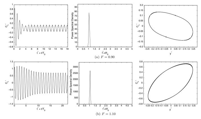
Fig. 9. Time series of the fluctuating lift coefficient  $C'_{\rm L}$  (first column), PSD of the fluctuating lift coefficient (second column) and phase portraits (third column) for the cylinder forced to oscillate at F = 0.90 and F = 1.10.
