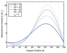
(b) Vorticity at the cylinder wall versus the angular position on the cylinder wall
