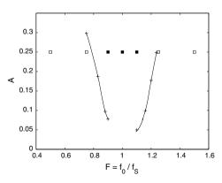
Fig. 8. Representation of the lock-in zone in the plane (A, F) for forced transverse oscillations. The solid lines represent the frontiers of the lock-in zone according to the data points (+) of Koopmann [24]. The simulations performed here are represented with squares: filled squares ( $\blacksquare$ ) correspond to locked configurations whereas empty squares ( $\Box$ ) indicate unlocked ones.
