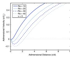
(a) Streamwise velocity versus the downstream distance after the cylinder wall
