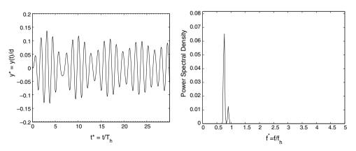
Fig. 18. Desynchronization of the cylinder oscillations at  $k_{\text{eff}}^* = 7.79$ : the peaks of frequency progressively shift from the values  $f^* = f_S/f_H = 0.68$  and  $f^* = 1$ .
