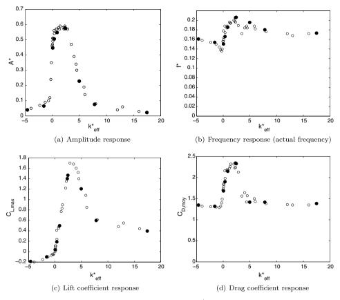
Fig. 15. Computed response ( $\bullet$ ) of the cylinder (amplitude *A* (a), actual frequency  $f^* = f_D/U_{\infty}$  (b), maximal lift coefficient  $C'_{L, max}$  (c) and mean drag coefficient  $\overline{C'_D}$  (d)) compared to the results of [40] ( $\bigcirc$ ).
