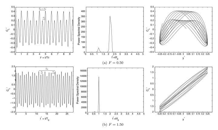
Fig. 10. Time series of the fluctuating lift coefficient  $C'_{\rm L}$  (first column), PSD of the fluctuating lift coefficient (second column) and phase portraits (third column) for the cylinder forced to oscillate at F = 0.50 and F = 1.50.
