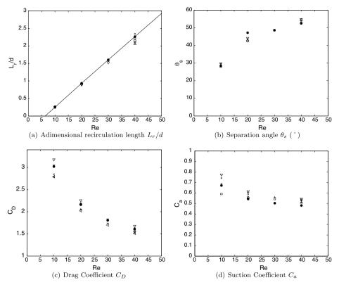
Fig. 4. Comparison of the geometric wake characteristics and aerodynamic force coefficients for the permanent regime (Re < 49). (•) present simulations, ( $\Box$ ) [16], ( $\Delta$ ) [5], ( $\blacklozenge$ ) [45], ( $\nabla$ ) [47], ( $\times$ ) [9], (+) [20,19], ( $\triangleleft$ ) [25].
