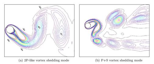
Fig. 14. Different vortex shedding modes obtained for (A, F) = (1.00, 0.90) (a) and (A, F) = (1.25, 1.50) (b).
