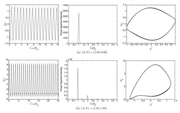
Fig. 13. Time series of the fluctuating lift coefficient  $C'_{\rm L}$  (first column), PSD of the fluctuating lift coefficient (second column) and phase portraits (third column) for the cylinder forced to oscillate at (A, F) = (1.00, 0.90) and (A, F) = (1.25, 1.50).
