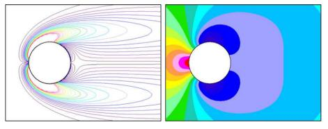
Fig. 2. Details of the vorticity contours (left) and pressure field (right) in the wake at Re = 40.
