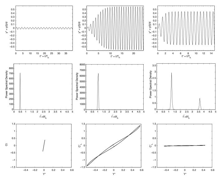
Fig. 16. Time histories of the cylinder displacement (first row), PSDs of the lift coefficient (second row) and phase portraits (third row) for VIV at Re = 100. From left to right:  $k_{eff}^* = 17.5$ , 2.32 and 0.05.
