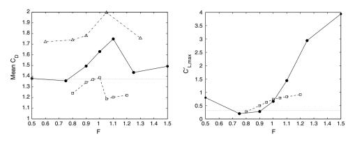
Fig. 12. Evolution of the mean drag and maximal lift coefficients with the frequency ratio *F*. The dashed lines give the values of the mean drag  $\overline{C'_{D}}$  and of the maximum lift coefficient  $C'_{L, max}$  for the fixed cylinder case. The results are compared to those of Anagnostopoulos [3] ( $\Box$ ) and Nobari and Naredan [29] ( $\Delta$ ).
