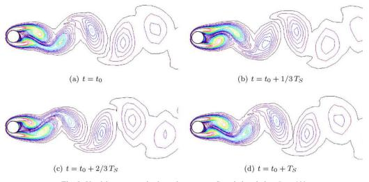
Fig. 5. Vorticity contours in the wake over one Strouhal period at Re = 100.
