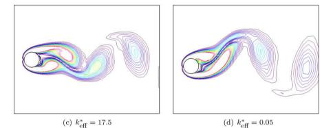
Fig. 17. Vortex shedding modes inside and outside the lock-in zone for the cylinder undergoing VIV at Re = 100.
