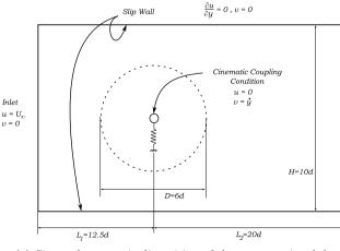
(a) Size and geometric disposition of the computational domain
