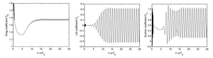
Fig. 6. Convergence of the aerodynamic fluctuating coefficients at Re = 100. From left to right: drag coefficient  $C'_{\rm D}$ , lift coefficient  $C'_{\rm L}$  and suction coefficient  $C'_{\rm a}$ .
