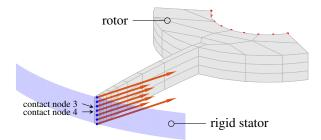
Fig. 1: Simplified finite element sector. Contact nodes [•], constrained nodes [•], and corresponding contact forces [----].
