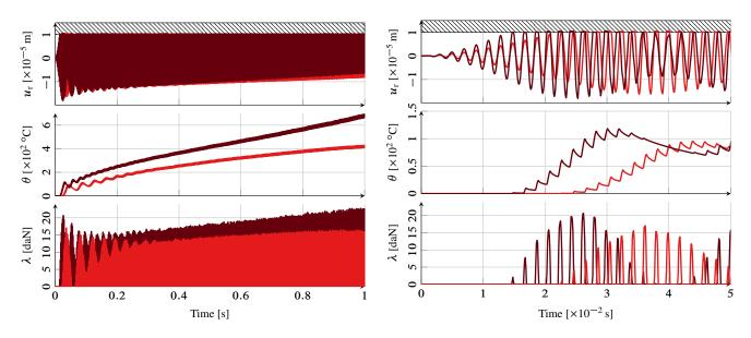
Fig. 12: Time histories for node 1. Effect of excitation amplitude: forcing of 1 [-] and 2 [-] normalized amplitude.
