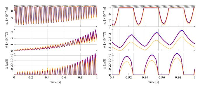
Fig. 2: Sensitivity to time-step in terms of radial displacement  $u_r$ , temperature  $\theta$  and normal contact force  $\lambda$  at node 4. Reference [-],  $h = 10^{-4}$  s [-] and  $h = 10^{-5}$  s [-].
