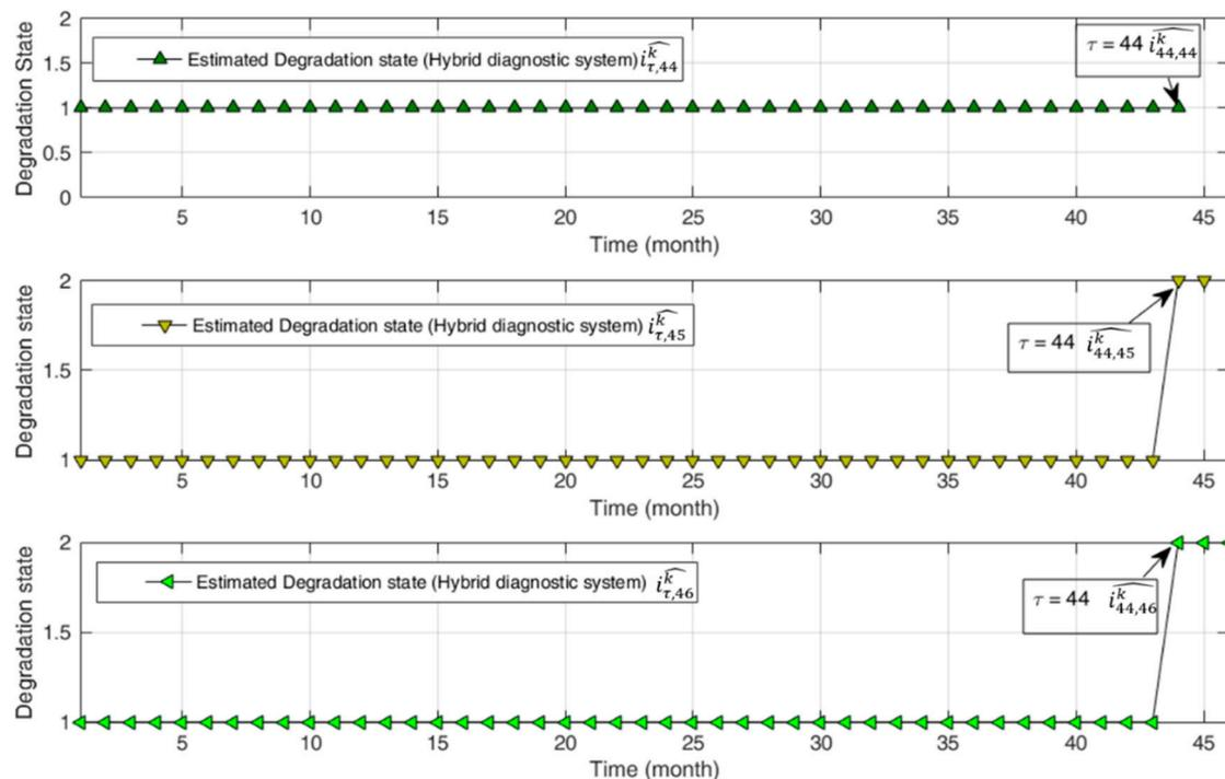
**Figure 8.** Estimate of the degradation state at time  $\tau = 44$  performed using the observation collected until time  $t = \tau = 44$  (top),  $t = 45$  (middle), and  $t = 46$  (bottom). Notice that at time  $t = 45$ , the hybrid method is able to correctly classify the component state.
