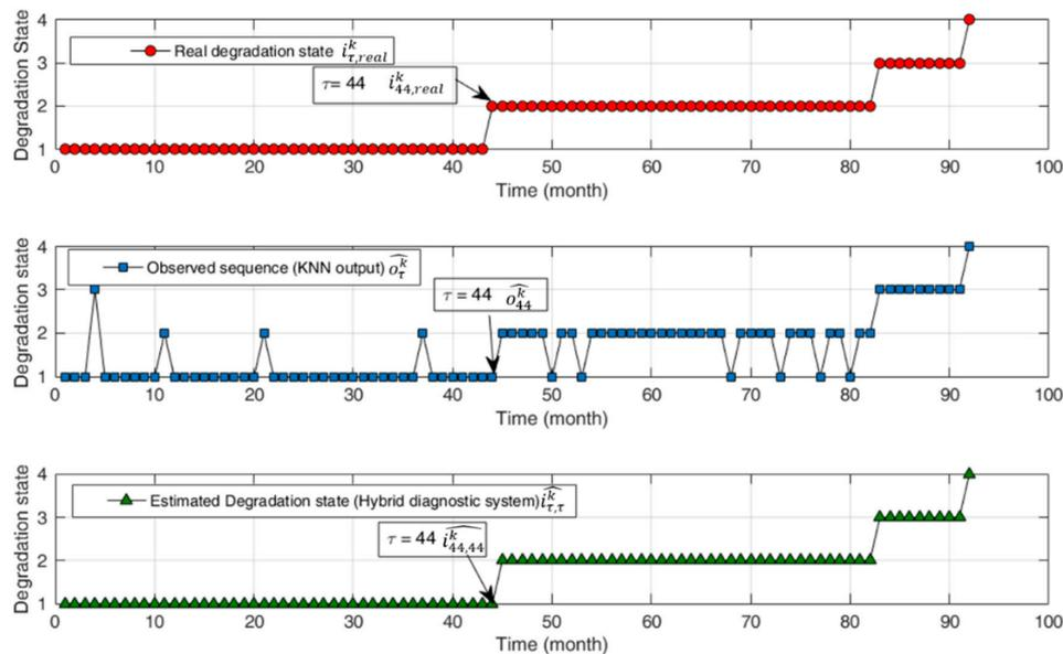
**Figure 7.** Typical case in which degradation state errors occur (**Top:** real degradation states; **middle:** degradation states estimated by the KNN classifier; **bottom:** degradation states estimated by the hybrid diagnostic system).
