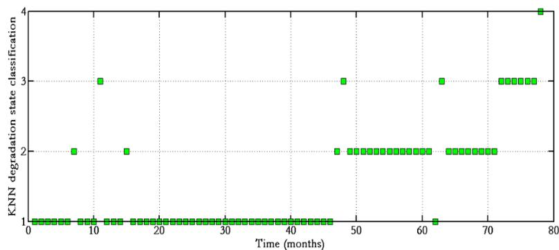
**Figure 4.** Classification of the degradation state during the degradation trajectory of Figure 3. The true degradation state of the component is state 1: from 0 to 46, state 2: from 46 to 71, state 3: from 72 to 77, and state 4: at time 78.
