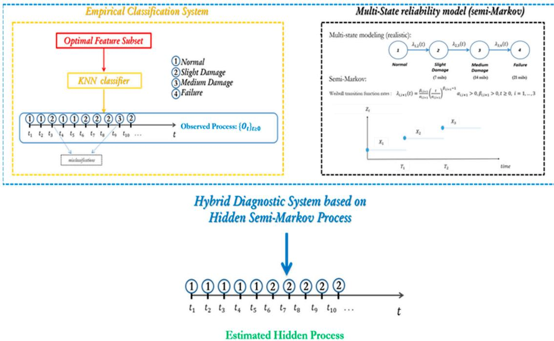
**Figure 1.** The hybrid diagnostic system based on homogeneous continuous-time finite-state hidden semi-Markov (HCTFSHSM). In particular, we set the entries of the observation matrix  $B$  as the estimated misclassification probabilities of the KNN classification algorithm.
