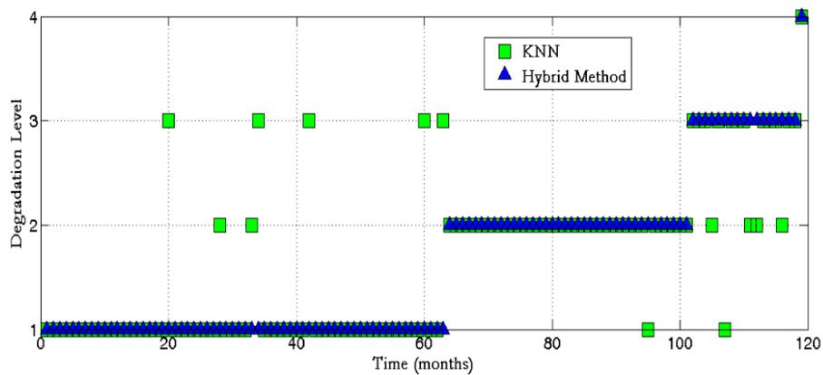
**Figure 6.** Example of observed sequence (squares) and estimated degradation state sequence (triangle). The true degradation state of the component is state 1: up to time 64 months, state 2: from time 65 to time 101 months, state 3: from time 102 to time 118 months, and state 4: at time 119 months.
