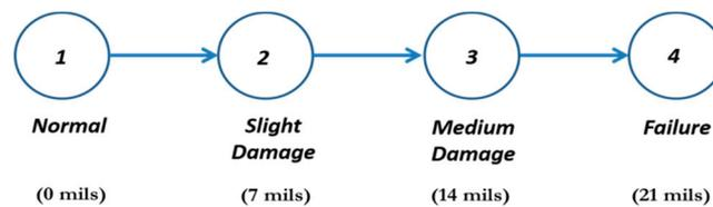
**Figure 2.** Four-state (left-to-right) model for the degrading bearing.
