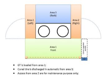
Fig. 9. Layout of the curing machine.
