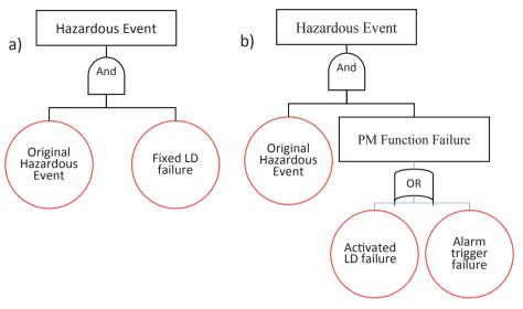
Fig. 3. Fixed devices (a) and activated devices (b).
