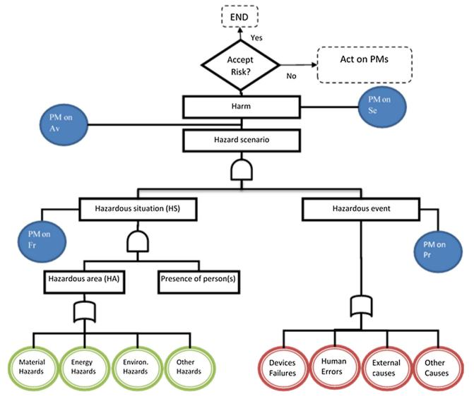
Fig. 1. Synoptic of hazard analysis.
