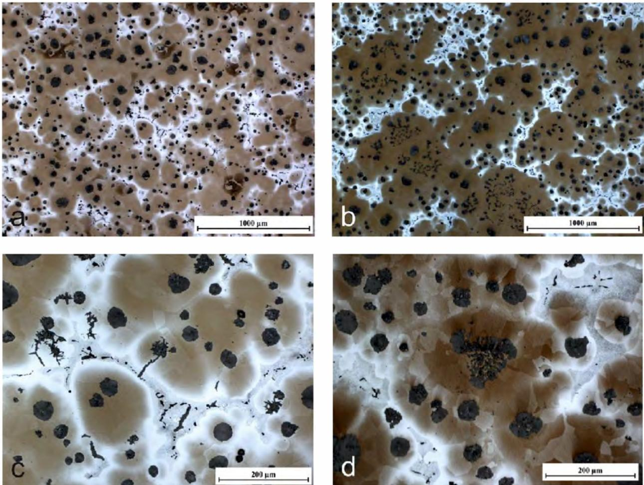
Figure 3: NaOH+CrO<sub>3</sub> etched micrographs of the samples SG-Pb (a and c) and SG-PbCe (b and d). The last to freeze regions appear bright coloured
