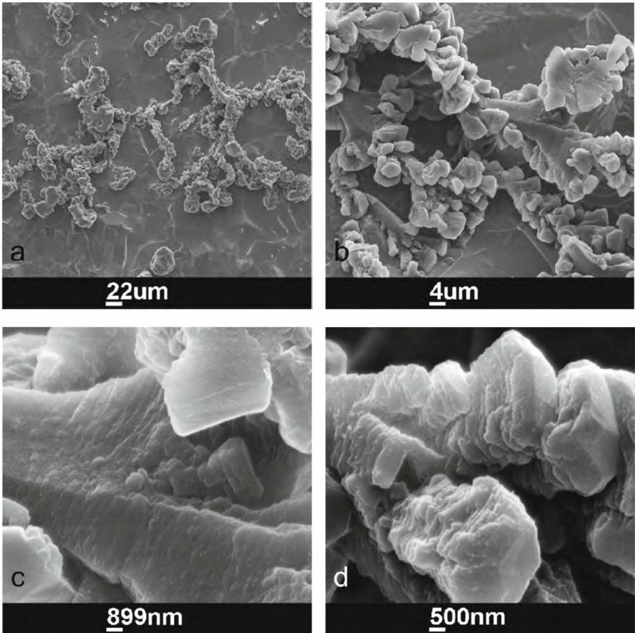
Figure 7: Chunky graphite in deep etched SG-PbCe sample
