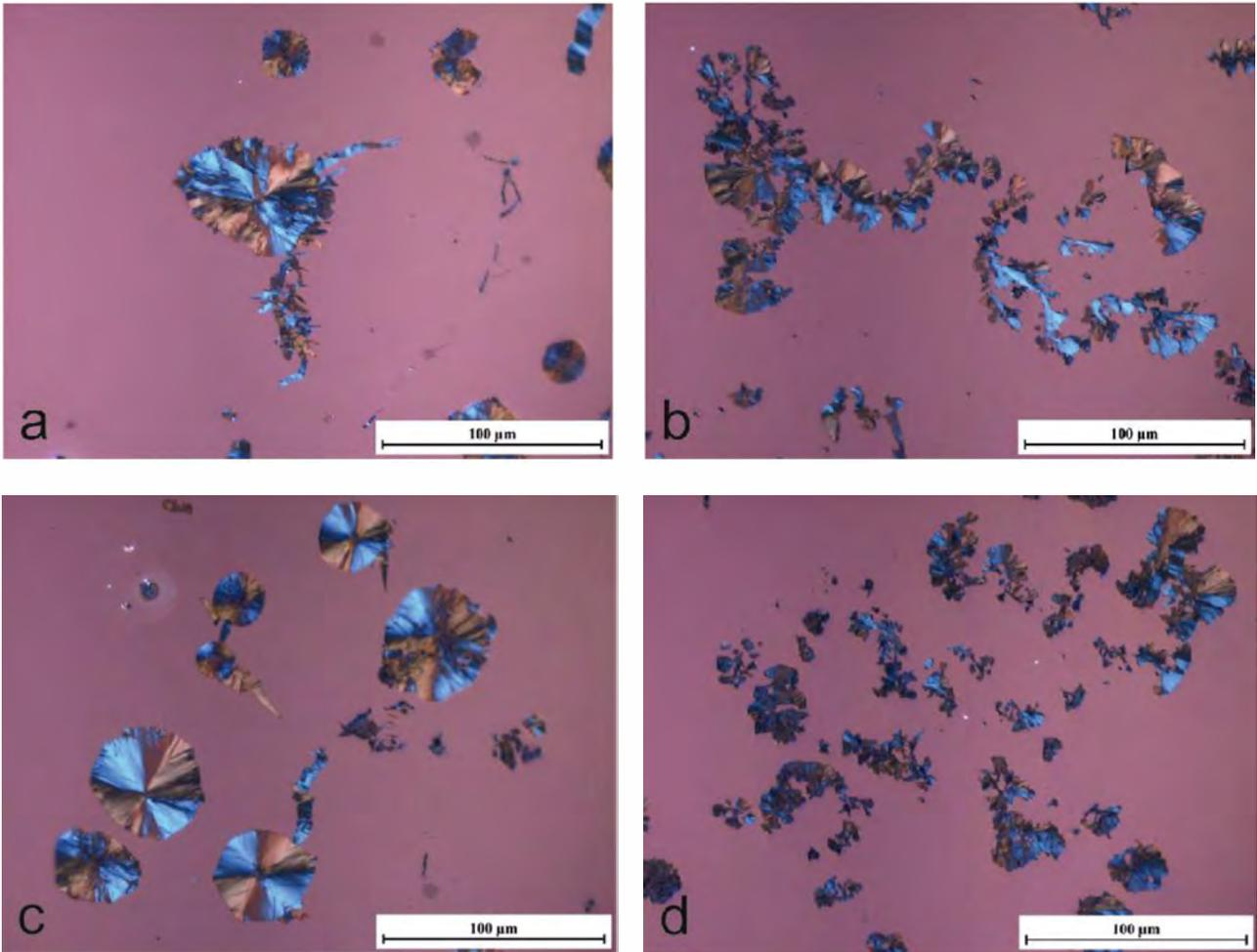
Figure 4: Graphite morphology under polarized light of sample SG-Pb (a and c) and sample SG-PbCe (b and d)
