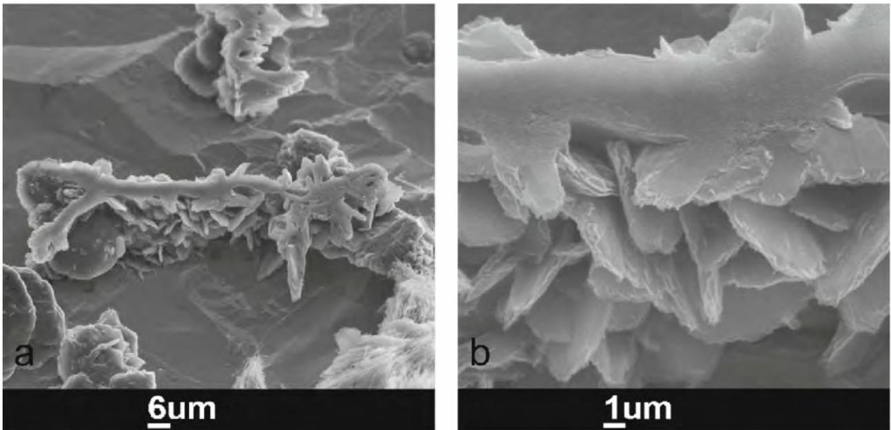
Figure 6: SEM micrographs of a graphite flake in deep-etched SG-Pb sample (a) and enlargement of the central part of the flake (b)
