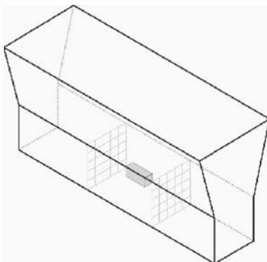
Figure 1: Y4 sample with sampling point for microstructure analysis
