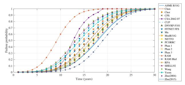
Figure 8: Failure Probability comparison for the selected models
