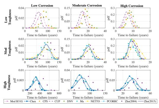
Figure 9: Probability density function of the time to failure per corrosion rate and material toughness
