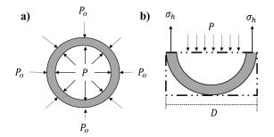
Figure 1: Free Diagram pressurized pipeline. Adapted from [34].
