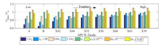
Figure 6: Flow-to-ultimate stress ratio comparison
