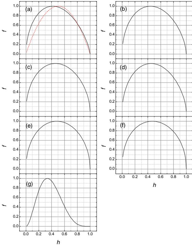
Fig. 4. Variation of the pinning force scaling  $f$  vs.  $h$  with position, samples (a)–(g). In all cases, the final fit to all scaling data is shown. The peak positions,  $h_0$ , are found to vary between 0.45 and 0.5, with the exception of strut (g), where a peak position of  $h_0 = 0.33$  is obtained. For the peak positions and the scaling parameters, see Table I. The dashed red line in panel (a) is the DH pinning function with  $p = q = 1$ .
