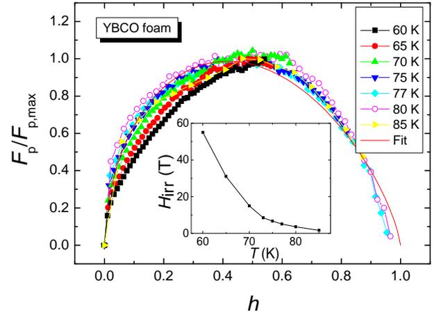
Fig. 3. Pinning force scaling,  $f = F_p/F_{p,max}$  vs.  $h = H_a/H_{irr}$  of foam strut (a). The red line presents the fit function to all experimental data shown. The inset gives the irreversibility line,  $H_{irr}(T)$ , as determined from the closing of the hysteresis loops and adjusted by the scaling.
