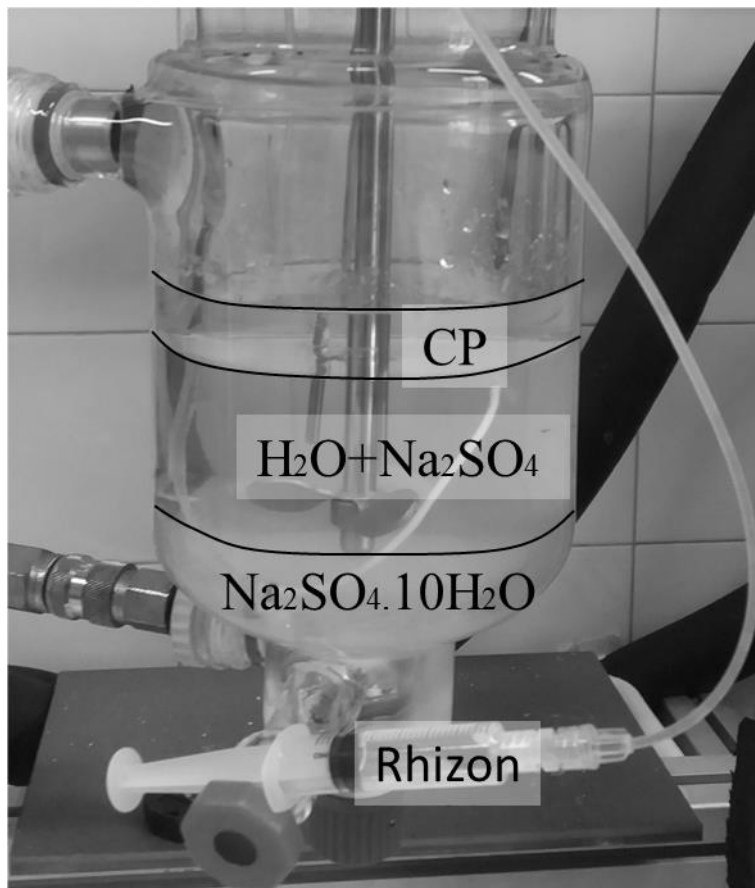
Figure 4. Photo of the experiment with Na 2 SO 4 at 8%, 5.4°C following the slow procedure.
