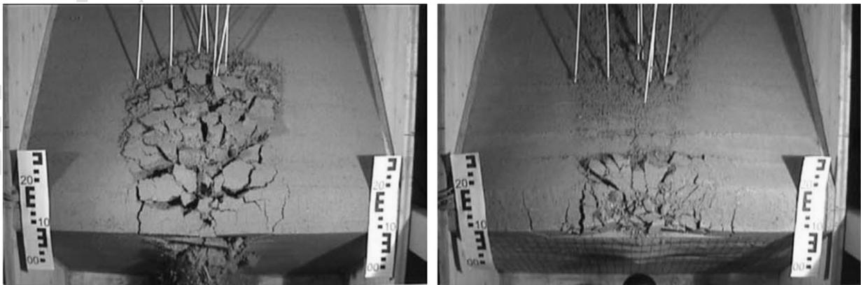
Fig. 7. Post-impact top views of small-scale embankments showing the influence of the geotextile on the valley-side facing deformation: without/with geotextile, left/right. (From Brandl and Blosky, 2004).
