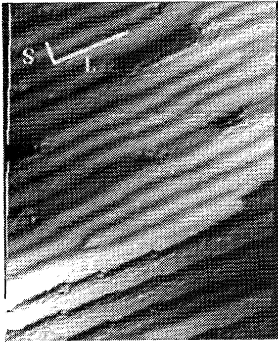
FIG. 1. 265 \text{ \AA} \times 300 \text{ \AA} image of the Au(100) surface prepared by ion bombardment ( \text{Ar}^+ , 600 eV, 10^{13} \text{ ions cm}^{-2} \text{ s}^{-1} , 40 s). A few vacancy islands slightly disturb the reconstruction which appears on the upper part of the image. Monoatomic kinked steps can be observed on the lower part. The "S" and "L" directions of the reconstruction are indicated.
