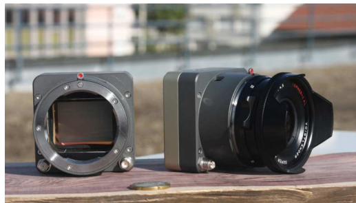
FIGURE 1: CamLight – the light metric camera for UAV applications developed at IGN.
