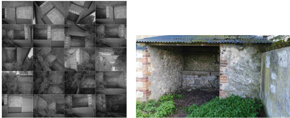
FIGURE 22: Images of the calibration field (left). The terrestrial calibration field used for pre-calibrating the camera (right).
