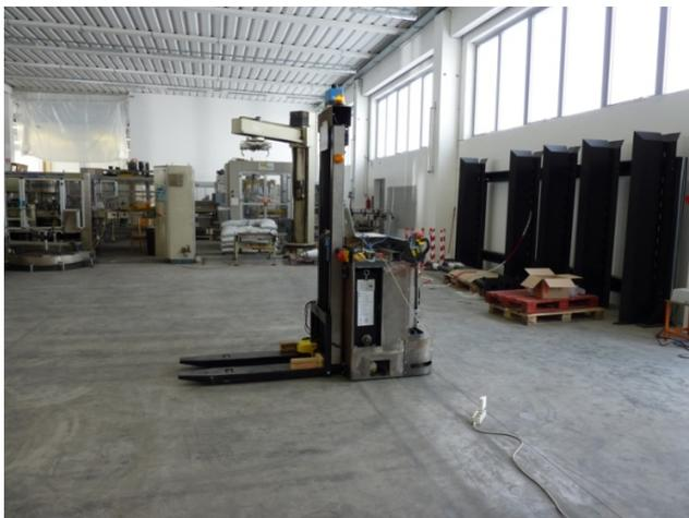
**Fig. 36 - A prototype of automatic guided vehicle**
