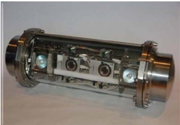
**Fig. 60 - TESSA: Stereoscopic camera for undersea archeological use**
