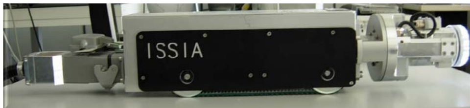
Fig. 78 - Prototype of mobile robot for non-destructive inspection of a multispar structure of Boeing 787
