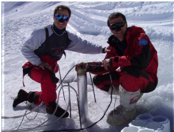
Fig. 63 - PANDORA a subglacial navigation robot designed by ENEA for Antarctica national program- tests on alpine glaciers
