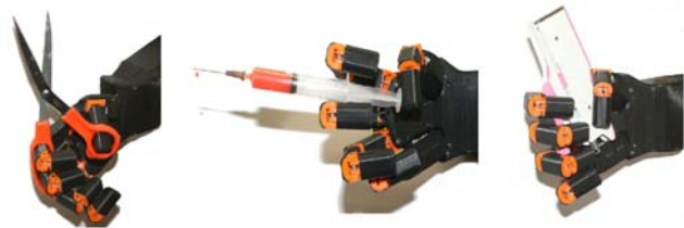
Fig. 49 - HE First Hand grasps trials: scissor (left side), syringe (middle) and stapler (right side)
