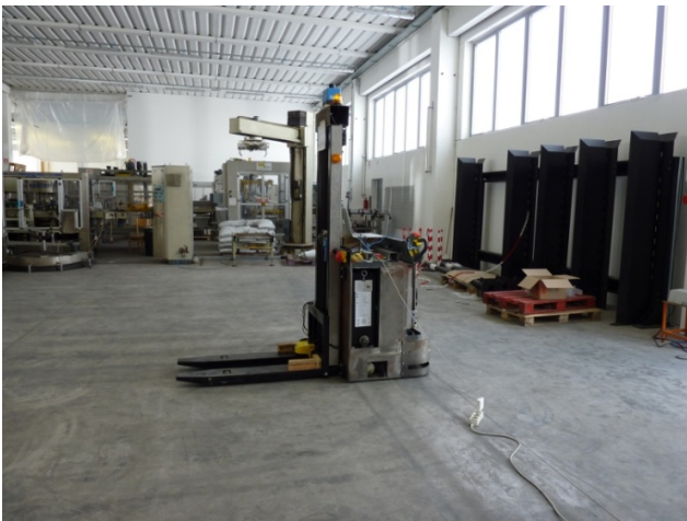
Fig. 36 - A prototype of automatic guided vehicle
