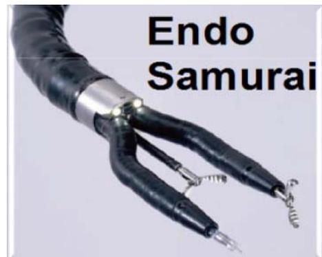
Fig. 29 - Endoscopic robot for surgery
