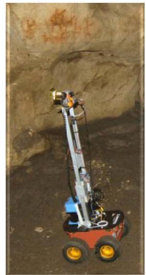
Fig. 77 - Robot used for cave exploration
