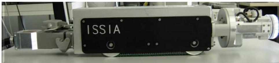
Fig. 78 - Prototype of mobile robot for non-destructive inspection of a multispar structure of Boeing 787
