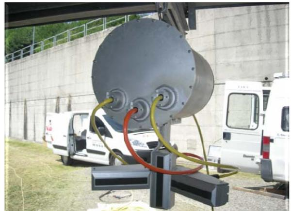
**Fig. 61 - STSS500 Ultrasonic stereoscopic 3D camera**
