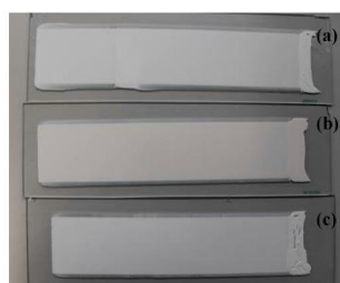
Figure 9: Films of waterborne paints (a) MOA-MMA; (b) commercial; (c) MLA-MMA
