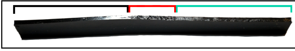
Fig. 6 Illustration of a pure shear specimen crack surface. The initial notch length appears in cyan, the rough surface due to steady crack propagation is marked in red and mirror-like smooth surface appears in black.
