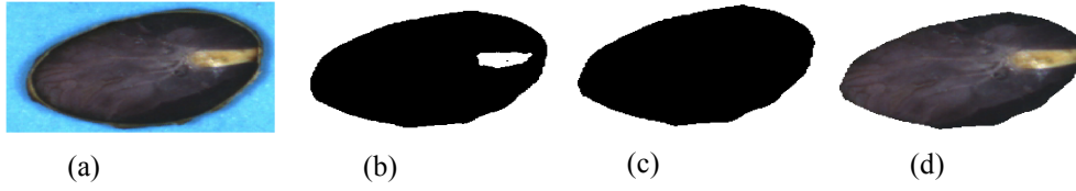
Fig. 4. Segmentation process: (a) Original image, (b) Otsu's thresholding, (c) Morphological opening, (d) segmented image
