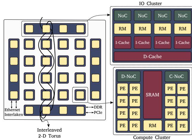
Fig. 1: Architectural overview of the Kalray MPPA-256 processor.
