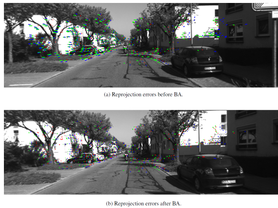
Fig. 9 Example of reprojection errors of the 3D points before and after BA, each color refers to the reprojection errors in a camera of the sliding window (5 images).
