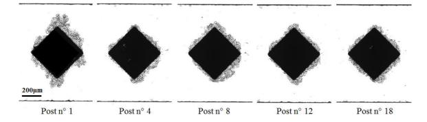
**Figure 7**: Bright field images of magnetically labeled cells captured on five different i-PDMS microstructure (post n°1, n°4, n°8, n°12 and n°18) in a microsystem integrating 20 i-PDMS microstructures
