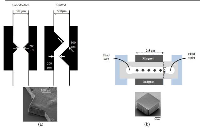
**Figure 2**: (a) DEP configuration in face-to-face and shifted designs featuring embedded C-PDMS electrodes, a SEM image is provided to show detail of the tip of the C-PDMS electrodes), (b) magnetophoresis configuration with i-PDMS diamond microstructures, a SEM image is provided to show detail of a i-PDMS microstructure.
