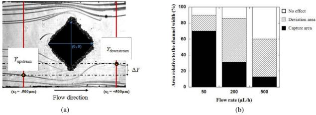
**Figure 6**: (a) Schematic representation explaining the measurement of the parameter  $\Delta Y = |Y_{upstream} - Y_{downstream}|$ . Y-positions of the beads were measured at two different locations : 500 µm respectively upstream  $(Y_{upstream})$  and downstream  $(Y_{downstream})$  from the center of the microstructure, allowing calculating the deviation of the bead, (b) Evolution of the measured deviation and capture areas as a function of the flow rate.
