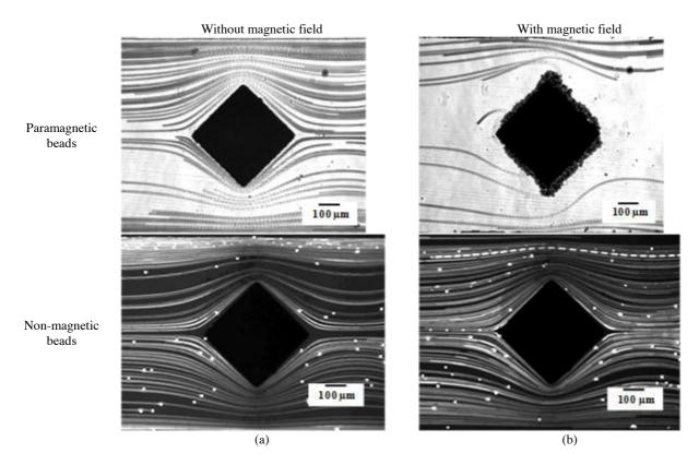
**Figure 5**: Z-stack projection of videomicroscopic images representing paramagnetic beads and non-magnetic beads flowing, under a flow rate of 50  $\mu$ L/h, at the vicinity of an i-PDMS microstructure in absence (a) and in presence (b) of an external magnetic field.
