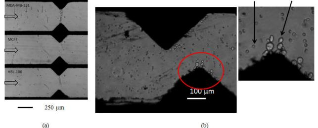
Figure 4: (a) Optical image showing three pairs of C-PDMS electrodes connected in bipolar configuration in three parallel microchannels used for cancerous cell lines capture using DEP (6.7 kV/cm at 1 MHz, 20  $\mu$ L/h), (b) optical image showing the capture of CTCs (MDA-MB-231) in RBCs flowing sample at 5  $\mu$ L/h (parameters were 0.75 kV/cm at 140 kHz). Microchannels were 100  $\mu$ m thick.
