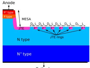
Cathode Fig. 1 – Schematic cross-view of the fabricated PiN diode.
