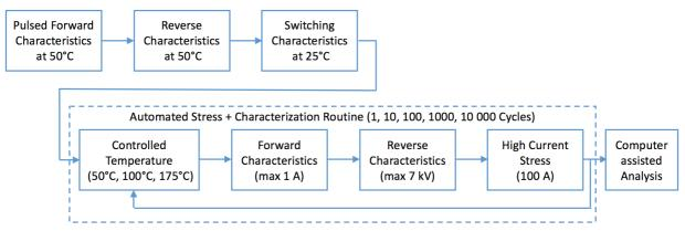
Fig. 3 - The specific characterisation procedure including the stress test that has been applied to the diodes.
