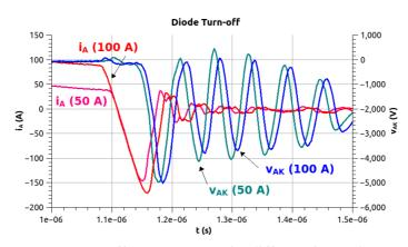
Fig. 6 – DPT turn-off measurements for different forward current  $i_F$  (50 A and 100 A) for a reverse applied voltage  $V_R$ =2.0 kV. The di/dt is clearly constant during the turn-off first phase with is classical in PIN turn-off.
