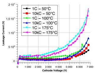
Fig. 10 – Reverse characteristics at increasing temperature after stress.
