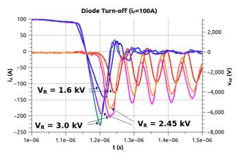
Fig. 7 – DPT turn-off measurements for different reverse applied voltage  $V_R$  (1.6 to 3.0 kV) for a forward current  $I_F$ =100 A.
