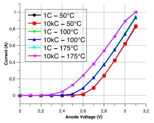
Fig. 9 – Forward characteristics at increasing temperature after stress.
