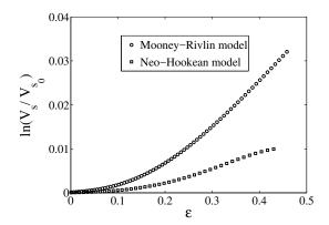
Figure 2: Total particles volume change  $\ln (V_s/V_{s_0})$  as a function of the cumulative vertical strain  $\varepsilon$ .
