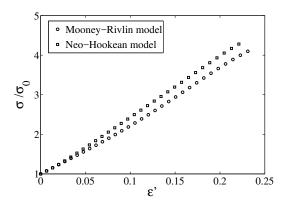
Figure 4: Normalized axial stress  $\sigma/\sigma_0$  as a function of cumulative strain  $\varepsilon'$  from the reference state defined by  $\sigma = \sigma_0$ .
