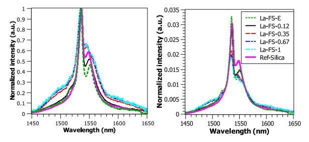
**Figure 6.** Maximum-normalized (**on the left**) and area-normalized (**on the right**)  $Er^{3+}$  emission spectra of lanthanum-doped samples. Samples are labeled according to their content in lanthanum;  $\epsilon$  is used for the sample where lanthanum content was too low to be measurable.
