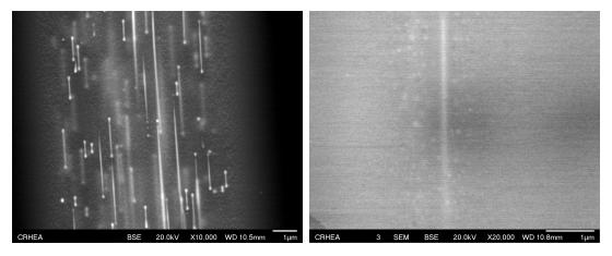
**Figure 3.** Secondary electron microscopy (SEM) images of the core of two optical fiber samples. The core sections correspond to the longitudinal view (along the drawing axis). The image on the left shows the core of the La-doped sample containing 1 atom % of La. The image on the right shows the highly doped part of the core of the Mg-doped sample containing 2.1 atom % of Mg.
