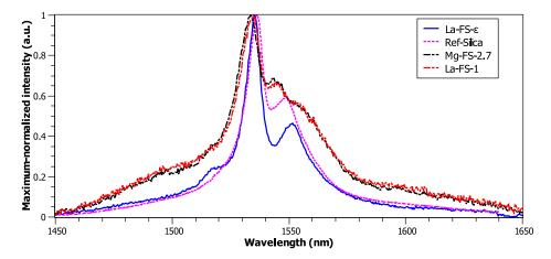
**Figure 7.** Comparison of the maximum normalization of  ${\rm Er}^{3+}$  emission spectra of the  $^4{\rm I}_{13/2}$  level in fiber samples. Emission spectra of highly doped Mg and La fiber samples are displayed with Ref-silica and low La content samples.
