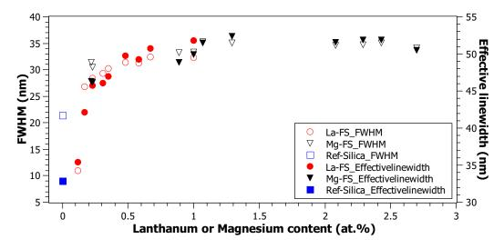
**Figure 9.** Evolution of Er<sup>3+</sup> emission bandwidth with lanthanum (black) and magnesium (red) content. Ref-silica values are shown in blue. Circle symbols are used for the effective linewidth (on the right scale) and crosses are used for FWHM (on the left scale).
