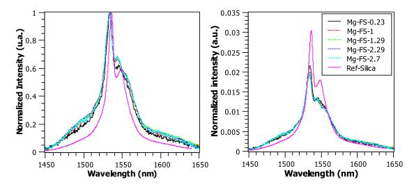
**Figure 5.** Maximum-normalized (**on the left**) and area-normalized (**on the right**) Er<sup>3+</sup> emission spectra of magnesium-doped samples. Samples are labeled according to their content in magnesium.
