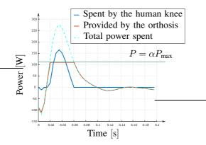
Fig. 3. Power of the knee at  $v = 1.0 \text{ m.s}^{-1}$  and  $\alpha = 0.4$ .
