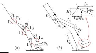
Fig. 1. Modelisation of the planed biped. a) Parameterisation of the biped. Note that angles are positive in counterclockwise. b) Length segments and position of the centers of mass.
