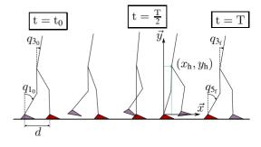
Fig. 2. A step of the biped and conditions of cyclicality.
